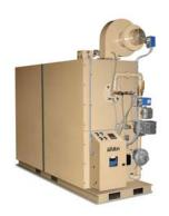
Fulton is launching a new 3,000,000 BTUH fully condensing hot water boiler with efficiencies up to 99% and modulation with a 5:1 turndown. It fits through standard door openings, has nearly zero standby losses and has no minimum return water temperature. This model is a direct vent/sealed combustion boiler, but it is not a pulse style.
