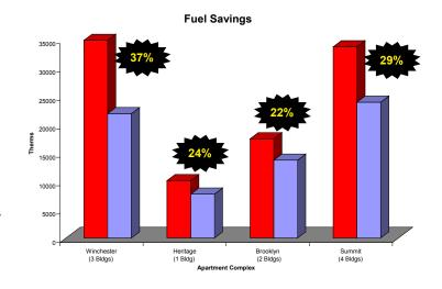
Four complexes (10 buildings located in Rochester, MN and Minot, ND) replaced their old cast iron boilers with Lochinvar Knight high efficiency boilers each having full modulating controls with 5:1 turndown. In addition, they replaced their tank style water heaters with Amtrol BoilerMates which are heated by the new Knight boilers. For the first 8 months, the buildings are seeing savings ranging from 19-45% with an average savings of 30%.
