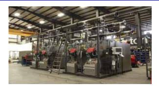
Mechanical Engineer: Wentz Associates Inc. Mechanical Contractor: Master Mechanical Equipment: Complete Package skid system -(4) Fulton Dual Fuel Vantage Condensing Boilers -
