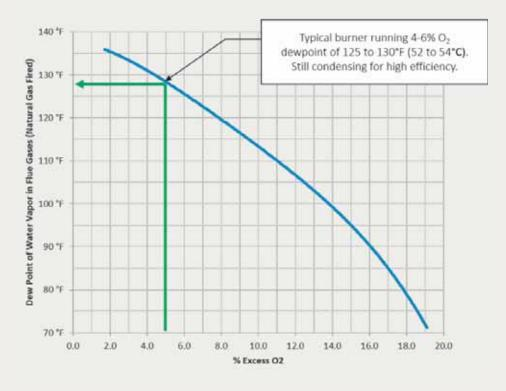
Every burner requires some excess air to maintain flame stability, ensure complete combustion, protect burner components, and limit emissions such as CO and NOx. The actual amount will vary, but for a typical natural gas burner found in a condensing boiler, you want this to be in the range of 4-8% O2 to allow for your boiler to actual condense.
