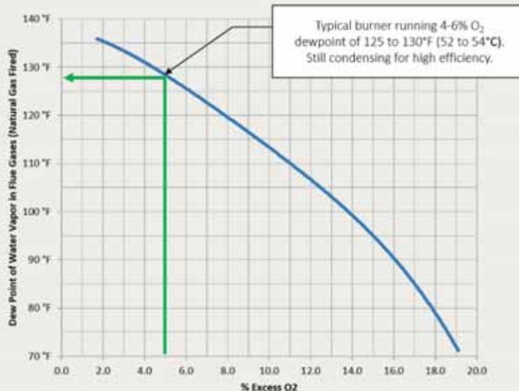
Every burner requires some excess air to maintain flame stability, ensure complete combustion, protect burner components, and limit emissions such as CO and NOx. The actual amount will vary, but for a typical natural gas burner found in a condensing boiler, you want this to be in the range of 4-8% O2 to allow for your boiler to actual condense.
