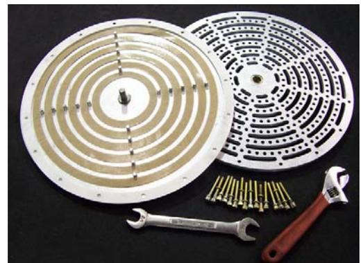
Now the assembly can be taken apart. Loosen the center adjustment screw and loosen until assembly comes apart. At this point, the air flapper gaskets and outer perimeter spacer will be exposed for cleaning or replacing.
