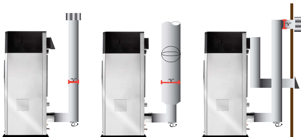
sidewall venting and combustion air inlet
